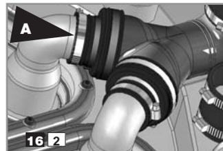
Unclip the cover. Unscrew the collar **A** on the faulty motor (the check valve stays in place while the motor is being repaired).
