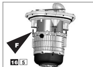
If the faulty motor has to be sent back to the manufacturer, you can operate the lifting station in minimum configuration with just one motor. Remove the screws **F** of the faulty motor from the inspection cover.
